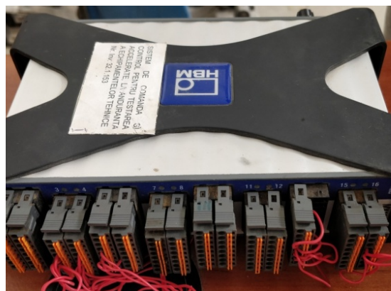
Fig. 4. HBM acquisition equipment
